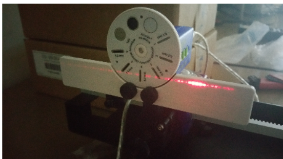
Figure 3: Single slit diffraction pattern. Rotate the slit accessory for height and alignment to achieve a pattern that is horizontal + centered on the slit in front of the light sensor.
